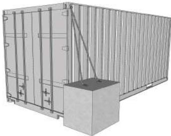
External ballast - pre-cast concrete block
