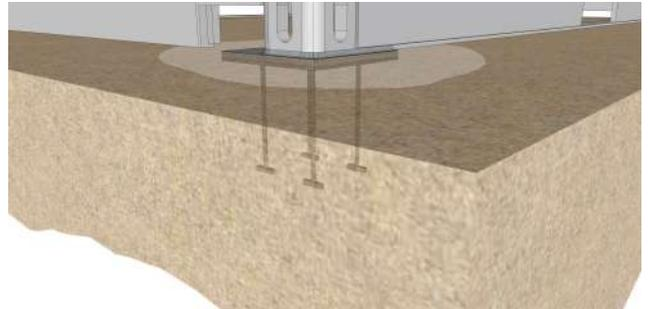
Concrete footing - welded container base plate
